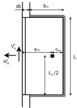
Horizontal component of weld stress
