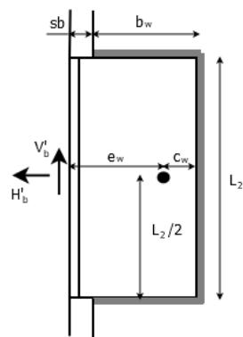
Horizontal component of weld stress
