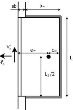
$$t_{wb,min} := \frac{2.0 \cdot 2 \cdot f_w}{0.6 \cdot F_{ub}}$$
