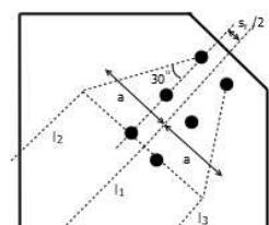
Buckling lengths along various points on the Whitmore section
