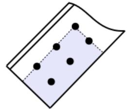
Interaction ratio in block shear
