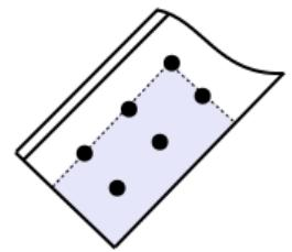
Interaction ratio in block shear
